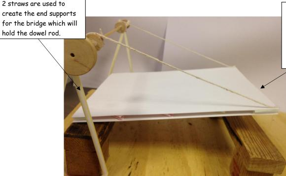
The system uses the dowel rod, pulley wheels and string to lift your reinforced paper bridge evenly and smoothly.
