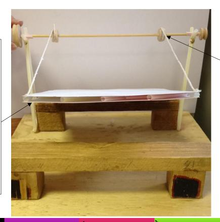
The string wraps around the pulley wheels, lifting the bridge.
